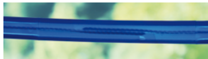
Upon completion of the welding process open the press and remove the profile.
