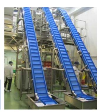
For special applications such as swan necks, the lugs can be positioned on the edges of the belt allowing full control in the critical bend of the conveyor.
